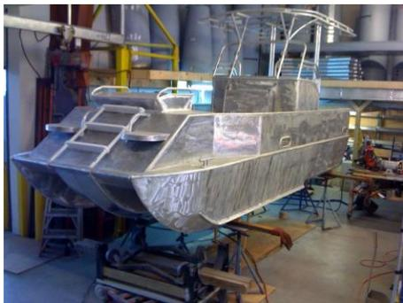
A new 22'-0" Aluminum Catamaran – Tender-Port Security-Sports Boat is completed, its solar powered(4) four panels total 1 kw with (2) torquedo 4.0 electric motors at 9.5 hp each, anticipated speed 14 knots.
